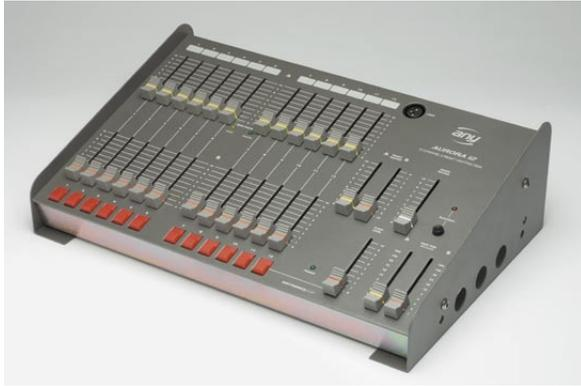
The Aurora 12 is a 12 channel 2 preset manual lighting desk designed primarily for schools and small drama groups. It is a low voltage unit, obtaining its power from the dimming packs to which it is connected. Apart from the expected features of "Blackout" and "Flash" switches, it does have a number of features normally only associated with more expensive desks, such as flash level slider, slaving facilities - even an optional gooseneck light.
